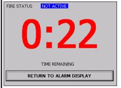
SINGLE ALARM PRE-DISCHARGE. NO-TICE THE FIRE STATUS INDICATOR. THE "RETURN TO ALARM MENU" WILL CHANGE TO "NEW ALARMS HAVE AR-RIVED" UPON THE DETECTION OF OTHER ALARMS.
