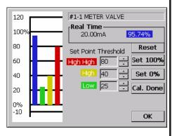
CONFIGURING A GAS INPUT. COLOR BARS INDICATE REAL TIME 4-20MA CURRENT AS A PERCENTAGE. SET POINTS ARE ALSO INDICATED.
