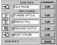
NAMING 4 INPUTS OF A NODE. EACH OF THE 4 CHANNELS HAS AN EDIT BOX TO WRITE MESSAGES FOR LAT-ER REFERRENCING.
