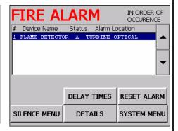
OPTIONS TO SELECT DURING AN ALARM. FURTHER OCCURING ALARMS WILL FOLLOW THE #1 ALARM INDICAT-ING ALARM. THE SCROLL BAR AL-LOWS SELECTIVE CHOOSING OF ANY ALARMS IN THE FIRE ALARM WINDOW. DELAY TIMES SELECTION BRINGS UP THE TIMING COUNTDOWN.
